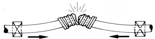
Effect of thermal expansion without guides.
